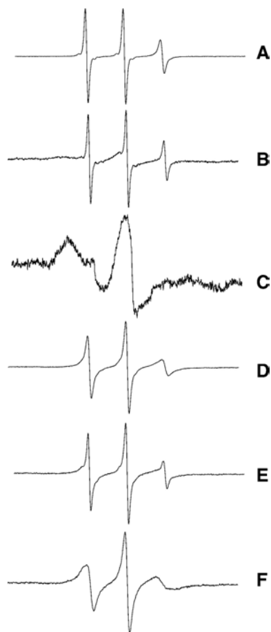
Fig. 2. EPR spectra of 0.1 mM [TOAC 1 ]-Gm: aqueous solution, (A); 1 mM SDS, (B); 5 mM SDS, (C); 10 mM SDS, (D); 5 mM LPC, (E); and 50 mM LPC, (F). The scan width is 100 Gauss.
